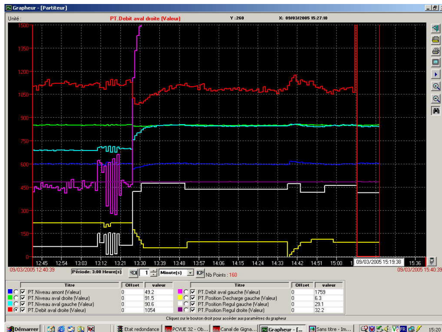
Figure 5. SCADA Display Showing an Autotuned ATV-PID Experiment
